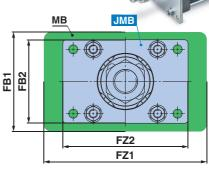
Width: Max. 20 % reduction, Height: 16 % reduction Dimension comparison (When mounted on the cylinder)
