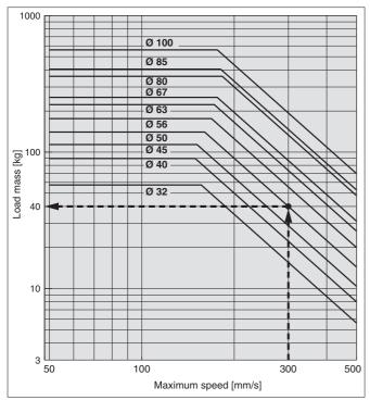
Example) Load limit at rod end when the air cylinder Ø 50 is actuated at 300 mm/s Extend upward from 300 mm/s on the horizontal axis of the graph to the intersection point with the line for a tube bore size of 50 mm, and then extend leftward from this point to find the load of 40 kg.
